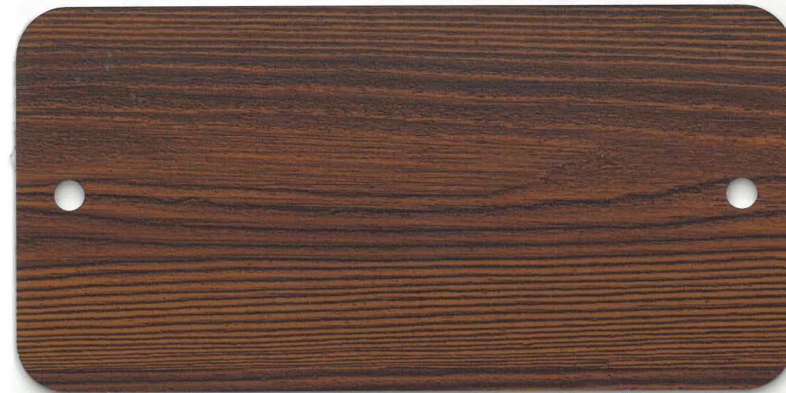
Powder Coating: DS 721 + Heat Transfer Film: 2117/02
