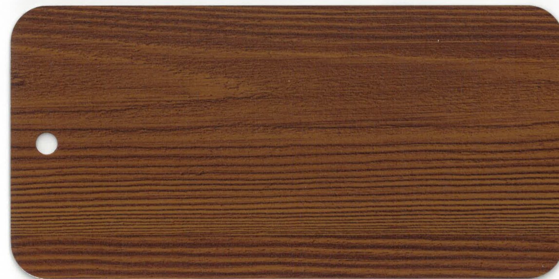
Powder Coating: DS 733 + Heat Transfer Film: 2117/12
