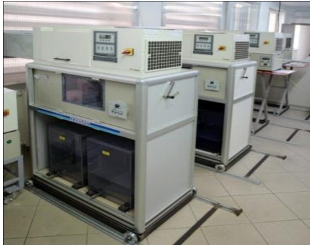
Pic 1: accelerated weathering test devices
