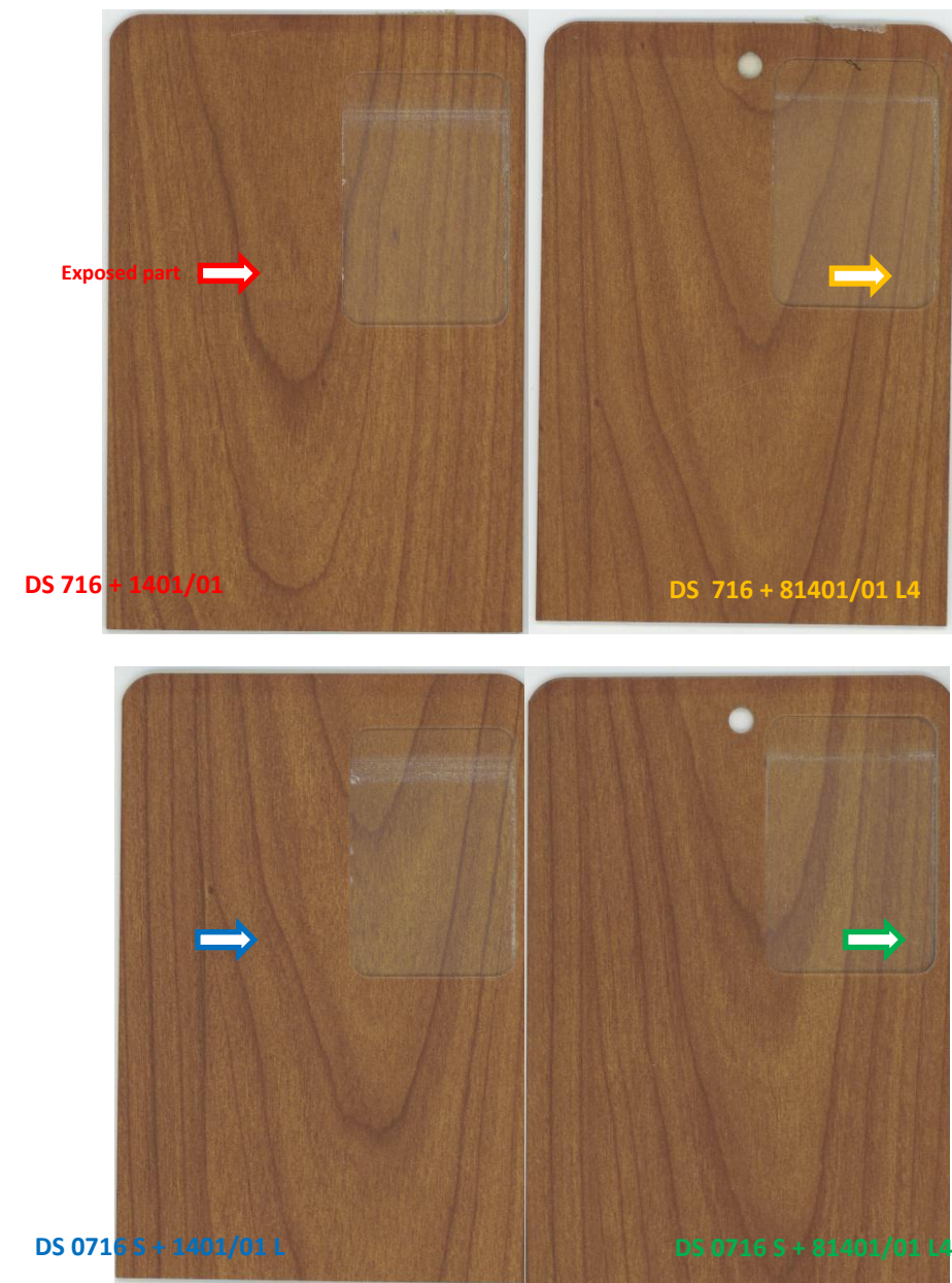
Pic 2: tested samples for 1000 hours (Standard powder) and 2500 hours (class 2 powder)
