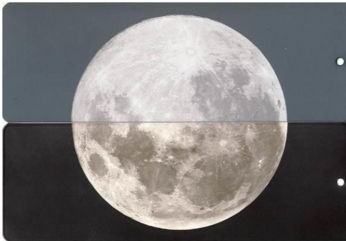
Figure 1: A picture of the moon, heat-transferred on one coat of DS 434 (upper panel) and two coats of PE411 + DS 407 (lower panel)
